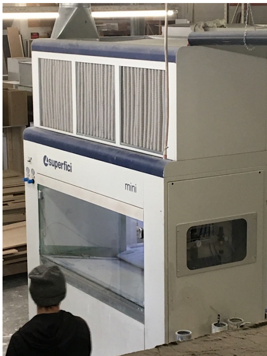
Superfici America Mini Plus spray machine in finishing area at Alka Kitchen Cabinets, Weston, Ontario, Canada
