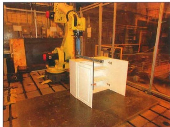
Figure 9 : Door fastening and hinge operation test set-up – Sample 3
