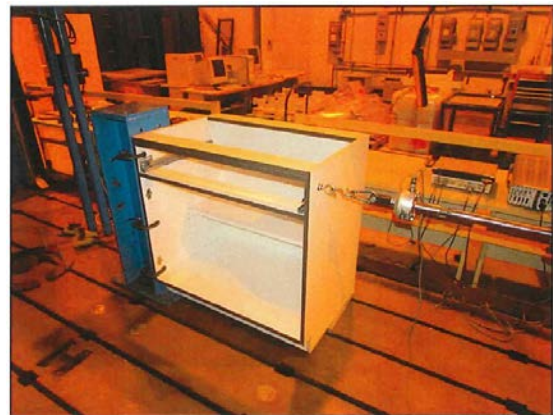
Figure 4 : Cabinet joint integrity test set-up – Sample 1
